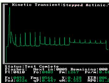
**Light curves:** Steady state photosynthesis at different levels of light intensity. Generation of light response curves using ultra stable actinic light source.
