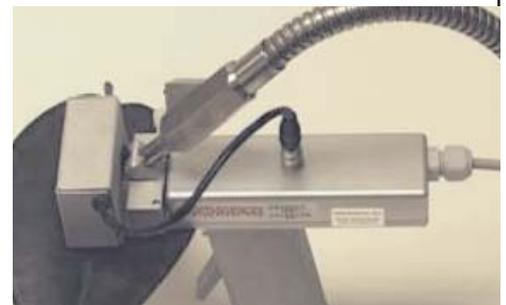
The Universal PAR Clip features a removable shroud with additional far red and blue photo diodes for the fluorescence identification of stress induced flavanoids. This technique enables UVA and UVB screening and Nitrogen Deficiency Testing (FRFex360/FRFex440).
