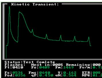
**Kinetic test:** Advanced quenching analysis using Puddle and Lake measuring parameters. Ultra stable light source ensures accurate measurements. NPQ, qP, qN and Y(II). Kramer lake model Y(II), Y(NPQ), Y(NO), and qL Hendrickson lake model Y(II), Y(NPQ) Y(NO) and NPQ.
