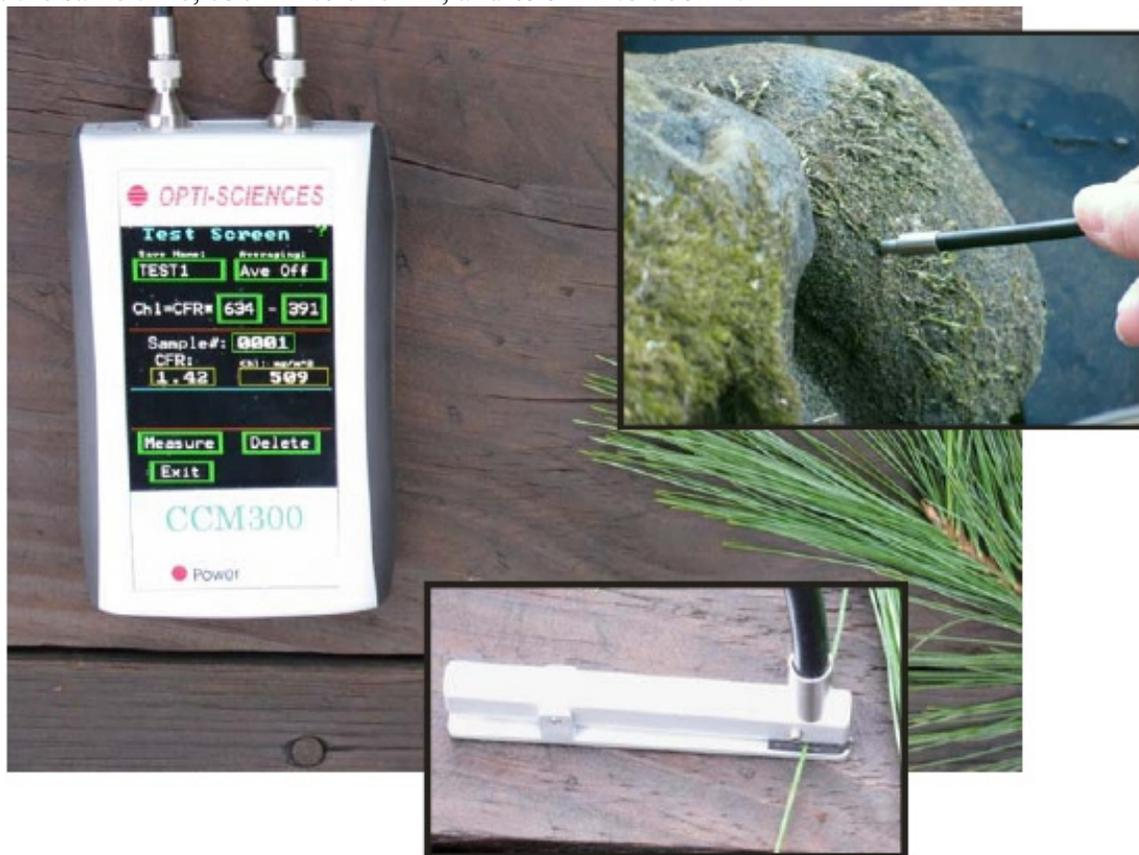
The instrument also provides two different readouts, one is the  $F735\text{nm} / F700\text{nm}$  ratio reported by Gitelson, and the other is a precise direct readout of chlorophyll content according to Gitelson's formula. The option also exists for changing formula parameters, incase a researcher should want to modify the formula for some unexpected, non-conforming plant species.
